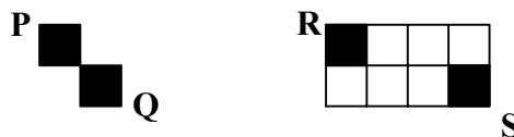
Figure 3. Left: Two neighboring points in the original image. Right: The corresponding points in the normalized image. The points in the rectangle are to be filled with black.
