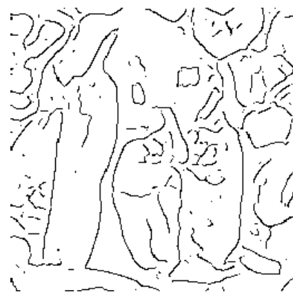
(f) Edge points from W_{2^2}^1 f(m, n) and W_{2^2}^2 f(m, n) using our method.
