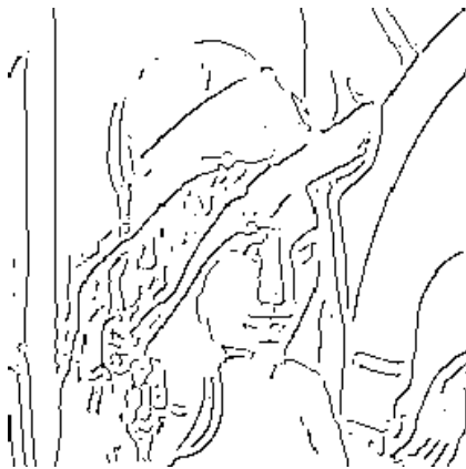
(e) Edge points from W_{2^3}^1 f(m, n) and W_{2^3}^2 f(m, n) using Mallat-Zhong's wavelet
