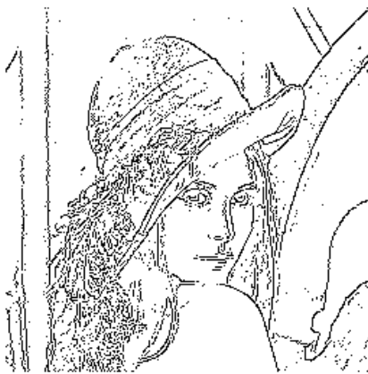
(a) Edge points from W_2^1 f(m, n) and W_2^2 f(m, n) using Mallat's wavelet .
