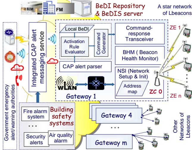
Fig. 8 Structure of BeDIS
