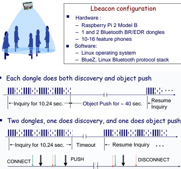
Fig. 6 Set ups for response time measurement
