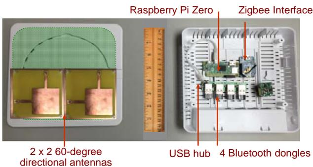
Fig. 5 Location beacons with dual-mode Bluetooth module
