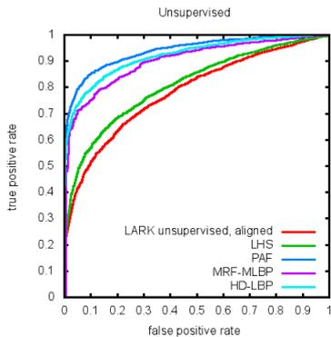
Figure 4: ROC curve of HD-LBP on LFW compared with other state-of-the-art methods under unsupervised protocol.
