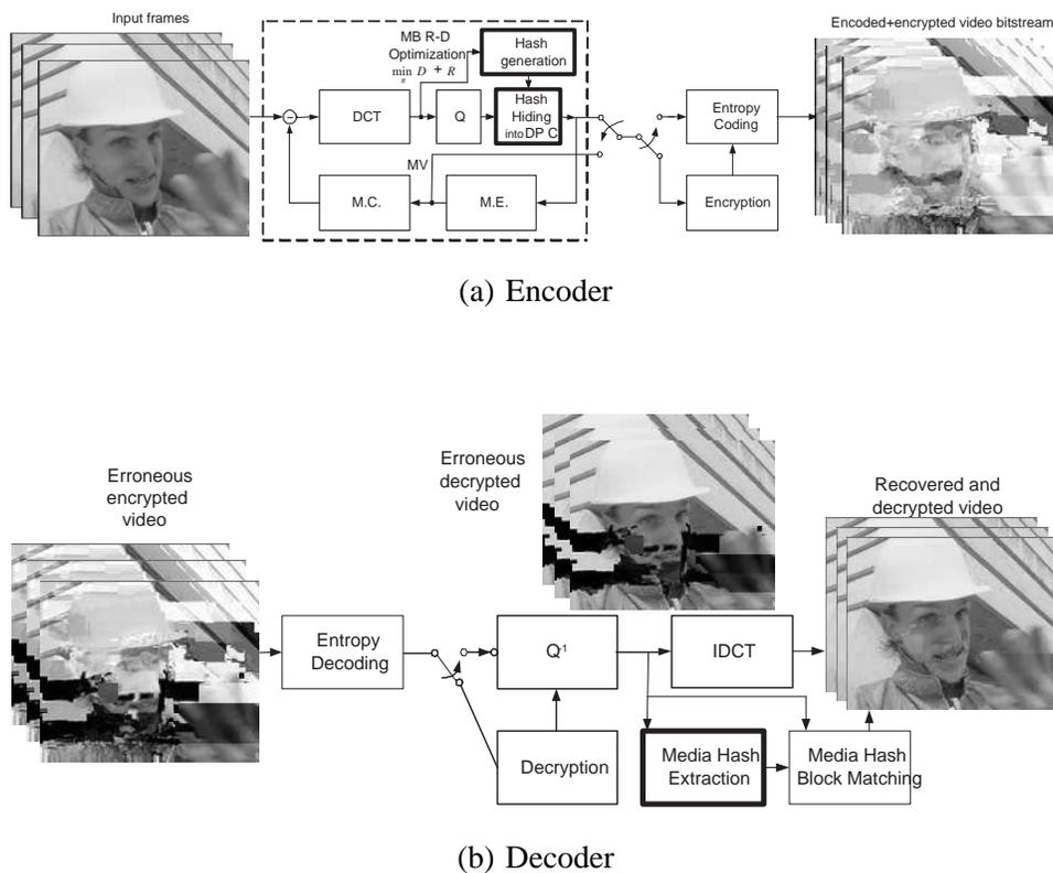
Fig. 7. Block diagrams of the proposed error-resilient video JET method: (a) Encoder; (b) Decoder.
