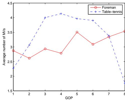
Fig. 17. The average number ( $n_{mv}$ ) of motion vectors in a macroblock for different GOPs.
