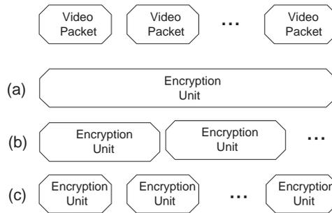
Fig. 8. **Different types of encryption unit: (a) all-in-one encryption; (b) desynchronization between video packets and encryption units; and (c) synchronization between video packets and encryption units.**
