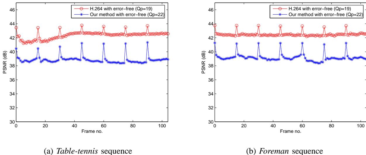
Fig. 11. PSNR comparisons before (H.264) and after (our method) data hiding: (a) *Table-tennis* sequence. (b) *Foreman* sequence. The bit rate is set to be 960 Kbps at encoder.
