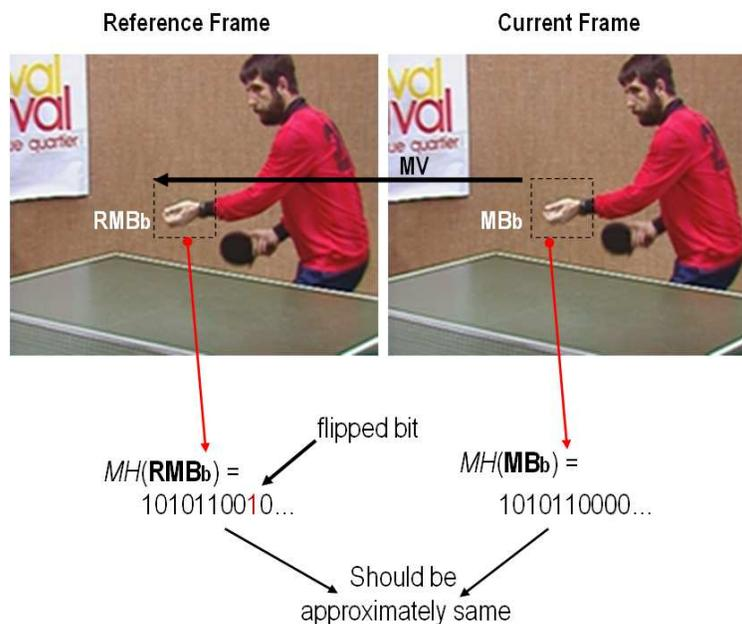
Fig. 6. The relationship between  $MB_b$  and  $RMB_b$ , and their corresponding media hash bits. If  $MB_b$  is lost, then the hash of  $RMB_b$  embedded in the residual data of  $MB_b$  can be extracted to find  $RMB_b$  for approximate recovery of  $MB_b$  because  $MB_b$  and  $RMB_b$  look perceptually similar.
