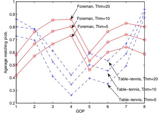
Fig. 18. The motion vectors matching probabilities ( $p_{cmv}$ ) in different GOPs.
